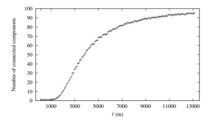
Figure 2: Average number of connected components in type-I networks as a function of the square side  $\ell$  for n = 100. All data points are averages over 1 000 network instances. Additional relevant parameters are P = 300 mW,  $N \approx 8 \times 10^{-14}$  W (for a bandwidth of 20 MHz at room temperature),  $\alpha = 4$ , and  $\beta = 25$  dB.
