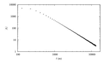
Figure 1: Average number of links in type-I networks as a function of the square side  $\ell$  for n = 100. All data points are averages over 1 000 network instances. Additional relevant parameters are P = 300 mW,  $N \approx 8 \times 10^{-14}$  W (for a bandwidth of 20 MHz at room temperature),  $\alpha = 4$ , and  $\beta = 25$  dB.
