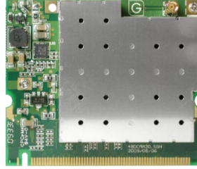
Figure 5: DSRC wireless mini-PCI module (DCMA-86P2 model) from Unex.
