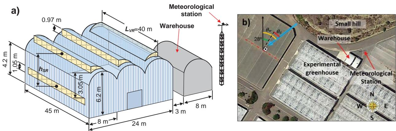
314 **Fig. 1.** (a) Dimensions of the experimental greenhouse and (b) neighbouring obstacles.
