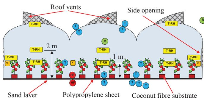
356 **Fig. 2.** Distribution of sensors located inside and outside the greenhouse for the measurement of climatic
