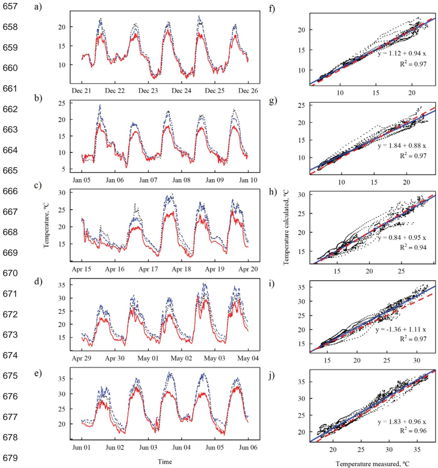
680 **Fig. 6.** Evolution of the outside  $T_e$  (—) and the inside air temperatures  $T_i$  measured (····) and calculated (- - -) in
