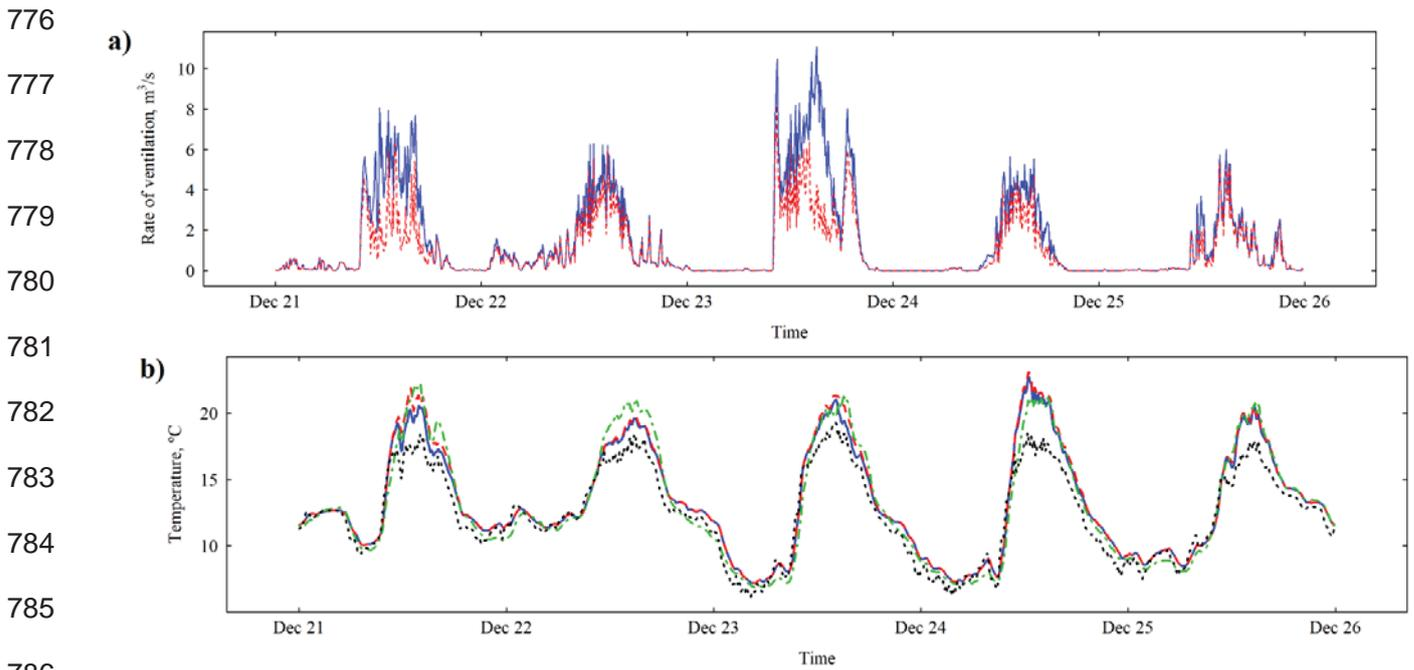
787 **Fig. 8.** Evolution of the ventilation flux  $G$  (—) calculated with Eq. (29) and corrected with the wind direction
