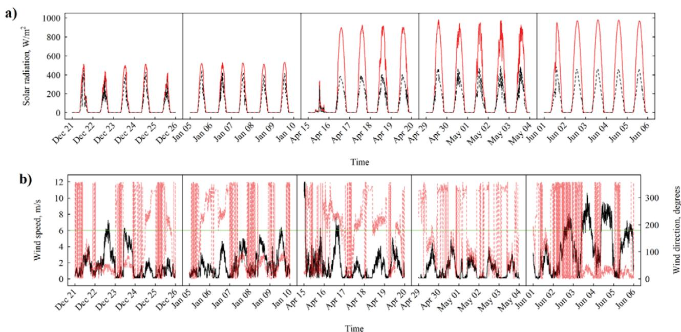
**Fig. 5.** Outside  $R_g$  (—) and inside  $R_{Si}$  (---) global solar radiation flux density during the five non-successive periods. (a). Evolution of wind speed  $U_0$  (—) and direction  $\theta_w$  (---) for the 25 days analysed, and wind-speed limit to begin to close windows (—) (b).
