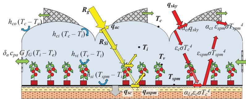
383 **Fig. 3.** Heat flux between the different components of the greenhouse model: solar (■) and thermal (■) radiations
