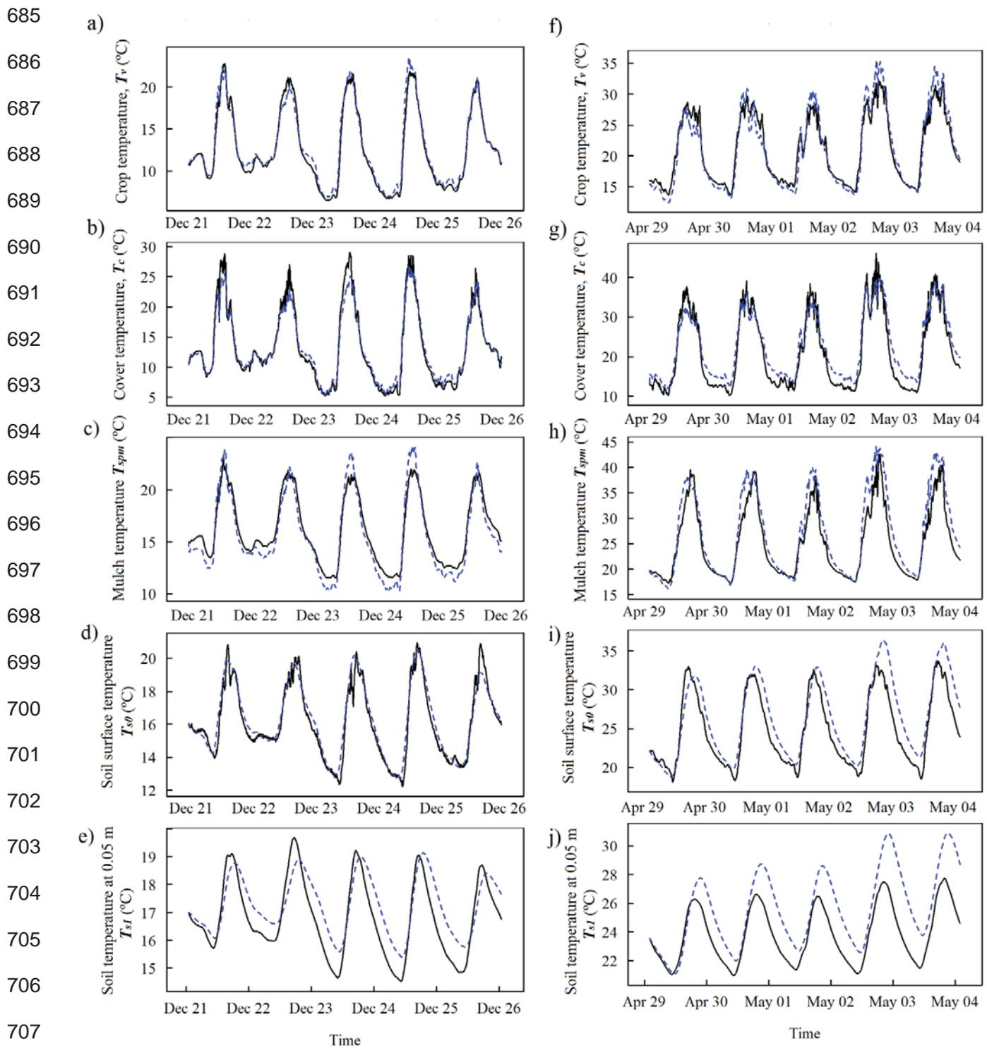
708 **Fig. 7.** Evolution of the measured (—) and calculated (---) values of temperatures of crop  $T_v$ , (a & f), greenhouse
