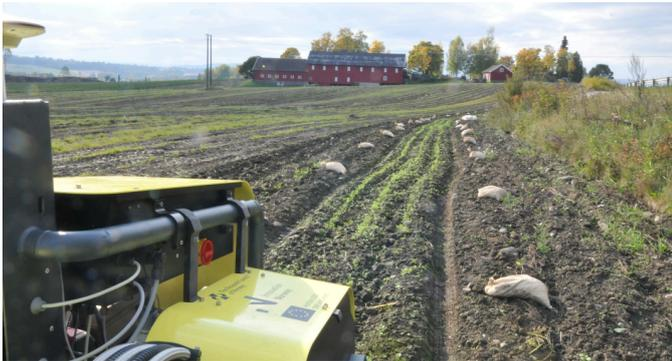
Figure 13: The robot at the start of the field trial. Only the center of the three carrot rows was used in the experiment.
