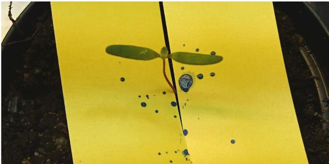
Figure 11: *Chenopodium album* L. after DoD application of liquid A3 with glyphosate. The liquid had very poor leaf retention properties, and satellite droplets were formed mid-air. No liquid is visible on the leaves, while the yellow liquid sensitive test strips highlight the droplets by turning blue. The droplets have either disintegrated in-air or bounced off the leaves.
