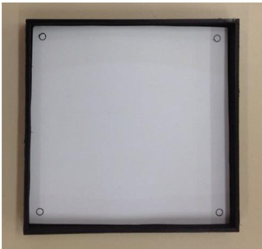
Fig. 3. Reference objects in image to calculate the size of aphids using a pixel per metric ratio.
