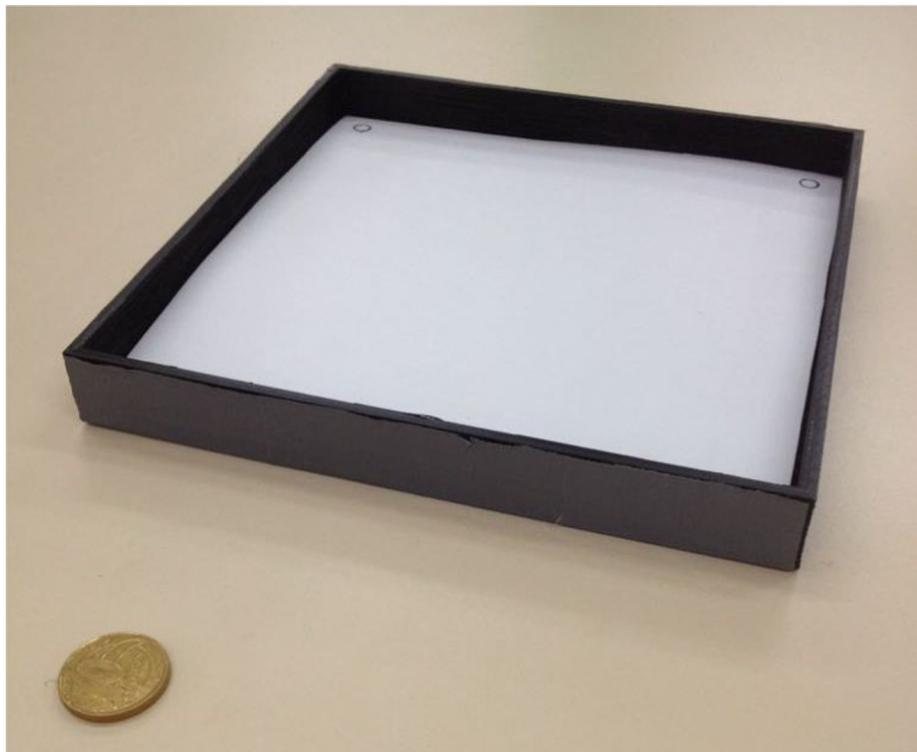
Fig. 1. Black-box used during image acquisition.
