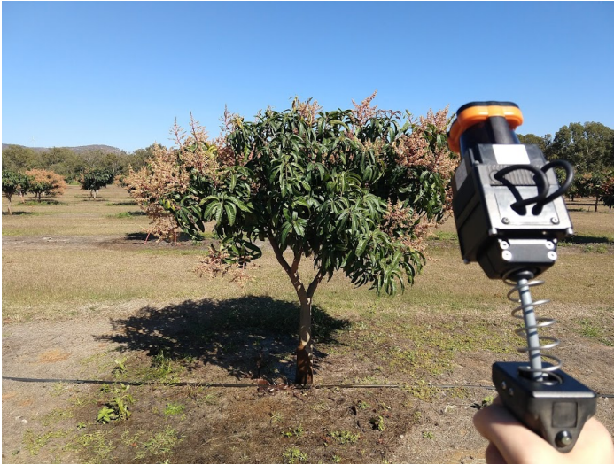
Fig. 2: GeoSLAM Zeb1 sensor scanning a young mango tree
