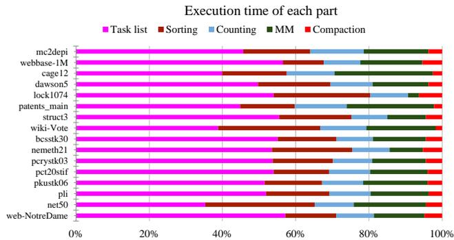
Figure 11: Relative runtime of the main parts of tSparse on Titan RTX.
