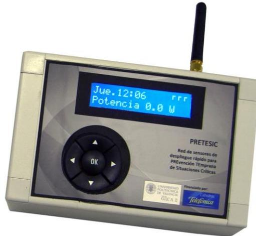
*Figure 9. Detail of a QSDN node. Sensors are attached to it via connectors on the left side*
