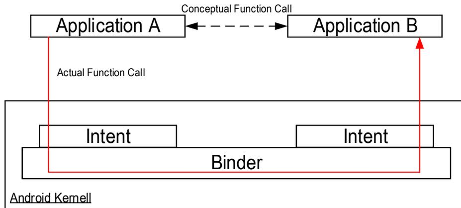
Figure 1. Inter-application Communication Using Android Intent and Binder
