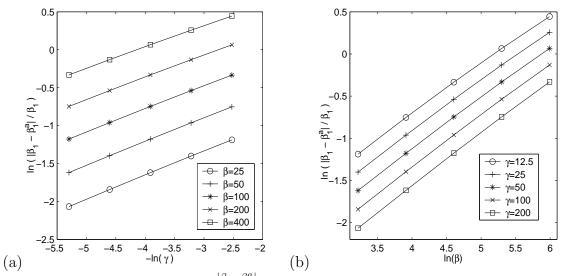
Figure 7: Convergence rate of  $\frac{|\beta_1 - \beta_1^a|}{\beta_1}$  for dimension reduction from 3D to 1D: (a) With respect to  $\gamma = \gamma_y = \gamma_z$ ; (b) with respect to  $\beta$ .
