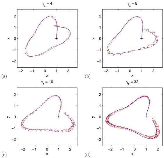
Figure 8: Trajectory of the vortex centers in 2D and 3D dynamics. Blue line (or flat curve):  $\mathbf{x}_{2D}(t)$ ; and red line (or oscillatory curve):  $\mathbf{x}_{3D}(t)$ .
