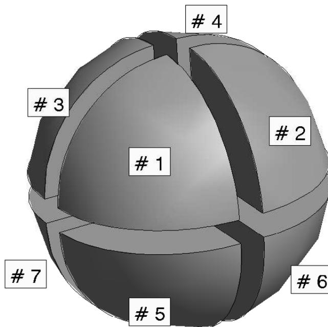
Fig. 2. Schematic view of eight-segment domain decomposition.
