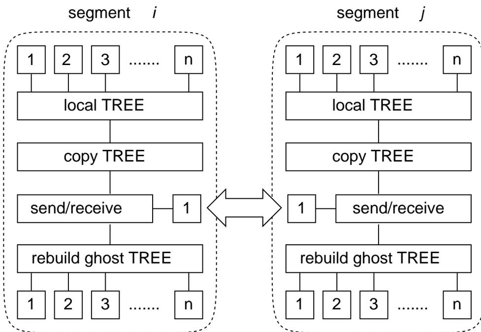
Fig. 4. Calculation and communication flow of each segment.
