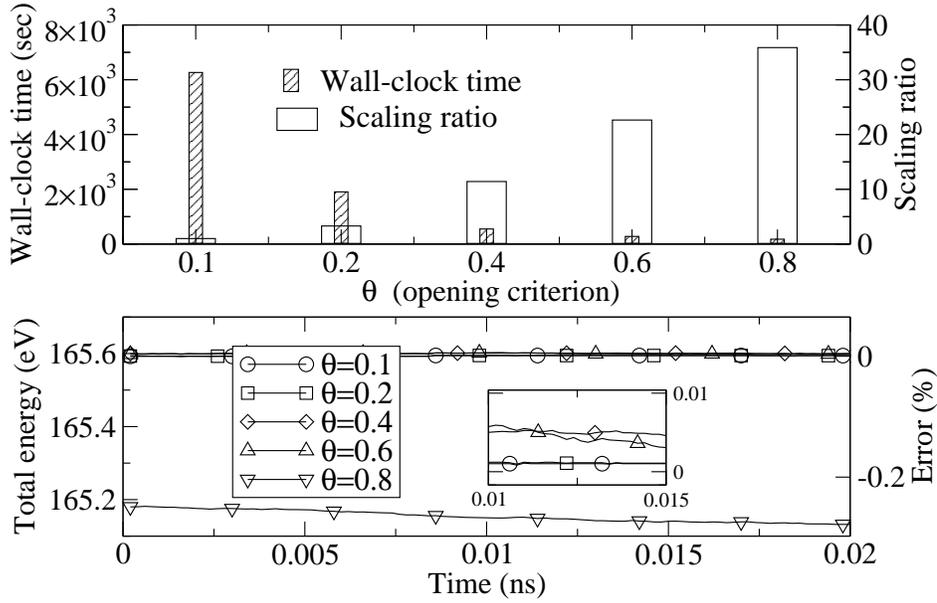
Fig. 9. Performance and energy curves in terms of opening criteria. Scaling ratios are the wall-clock time ratios with respect to  $\theta = 0.1$ , whereas the reference of error estimations was from all pair-wise calculations. The inset shows fine differences for  $\theta = 0.1 - 0.6$ , where x-axis is time (ns) and y-axis is error(%).
