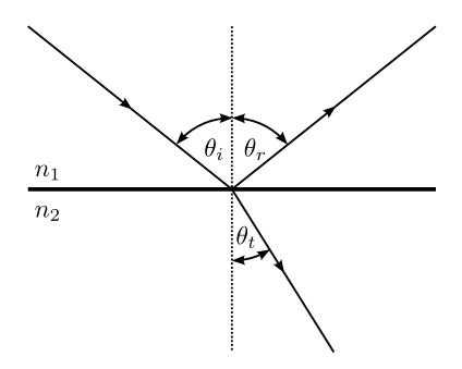
Figure 1: Reflection and refraction of light at a plane interface in the plane of incidence. The angle of refraction  $\theta_t$  is determined by the angle of incidence  $\theta_i$  and the refractive indices of both media  $n_1$  and  $n_2$  (Eq. 2). The angle of reflection  $\theta_r$  is equal to the angle of incidence  $\theta_i$ .
