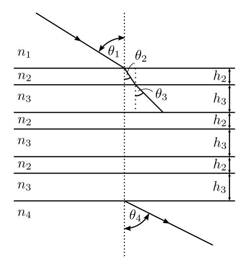
Figure 14: Scheme of a periodic multilayer. It consists of a stack of layers with alternating refractive indices,  $n_2$  and  $n_3$ , and thicknesses,  $h_2$  and  $h_3$  between two media with refractive indices  $n_1$  and  $n_4$ . Drawn here are only three periods, but the number of periods can be chosen arbitrarily. It is also possible to end with the transition from  $n_2$  to  $n_4$  skipping the last layer with refractive index  $n_3$ .
