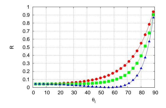
Figure 4: Reflectivity  $\mathcal{R}$  of a plane interface between homogeneous dielectric media with refractive indices  $n_1 = 1$  and  $n_2 = 1.52$  as a function of the angle of incidence  $\theta_i$ . Triangles: Polarization angle  $\varpi = 0$ ; Squares:  $\varpi = \pi/4$ ; Circles:  $\varpi = \pi/2$ . Each marker represents a simulation of 100000 events with  $\alpha = 0.99$ . The simulation data are in very good agreement with the wave theoretical predictions (solid lines).
