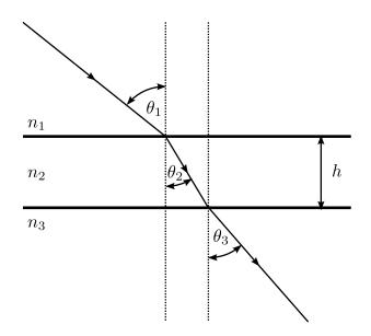
Figure 6: Homogeneous dielectric film built from two plane parallel interfaces. The film thickness is denoted by h. For a plate surrounded by air the refractive indices  $n_1 = n_3 = 1$  and  $\theta_1 = \theta_3$ .
