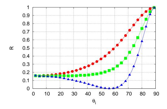
Figure 11: Simulation data of the reflectivity  $\mathcal{R}$  of a quarter wave plate as a function of the angle of incidence  $\theta_i$  for different polarizations  $\varpi$ . Triangles: Polarization angle  $\varpi = 0$ ; Squares:  $\varpi = \pi/4$ ; Circles:  $\varpi = \pi/2$ . The parameter  $\alpha = 0.99$  and 100000 events were processed for each data point. The simulation results (markers) are in very good agreement with the wave theoretical expressions (solid lines, Eq. (24))
