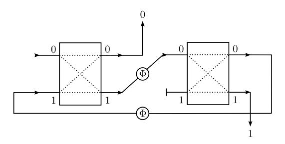
Figure 8: Arrangement of two DLMs simulating a homogeneous dielectric film. The output on port 0 of the second DLM is fed back into the input port 1 of the first machine. The symbol  $\Phi$  denotes a phase shift that a message acquires when travelling that specific path.
