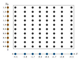
Figure 1: An example of a tensor product lattice. The specific unequal lattice spacing in the x direction is due to the fact that the basis functions in that dimension have been chosen to be Hermite-Gauss.
