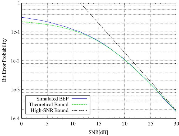
**Fig. 1.** Bit error probability of a 64-QAM with Alamouti code through a channel with Rayleigh fading ( $\sigma_{s,d}^2 = \sigma_{h,d}^2 = 1$ ).
