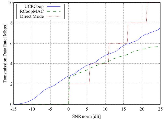
Fig. 2. Achievable data rates for different transmission modes: red-dotted for direct mode, green-dashed for RCoopMAC, and blue-solid for UCRCoop.
