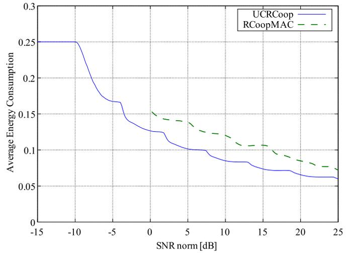
Fig. 5. Average energy per bit  $E_b$  transmitted at each relay node for both cooperative strategies: RCoopMAC and UCRCoop.
