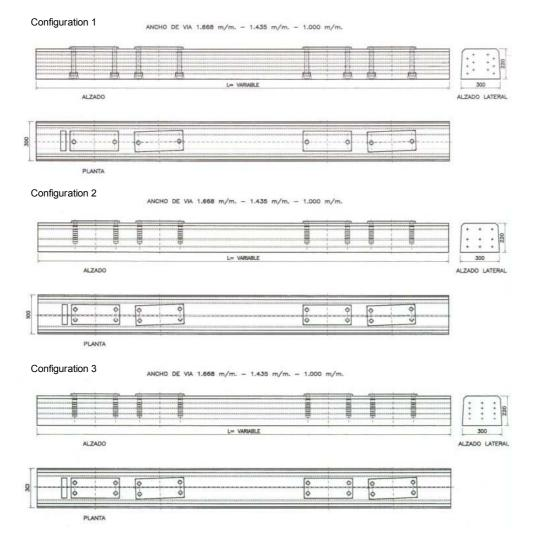
Figure 2: Configuration types (number and distribution of pre-stressed steel)
