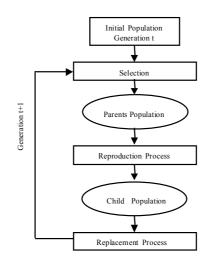
Figure 4. Simple flowchart of the genetic algorithm
