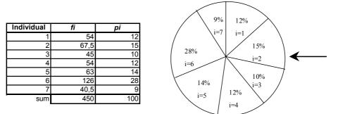
Figure 5: roulette wheel process selection.
