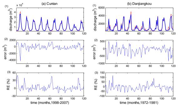
Figure 20. MA-ANN model results of one-day-ahead forecast for (a) Cuntan and (b) Danjiangkou. ((1) observed vs. predicted (2) error (observed – predicted) and (3) RE (representing Relative Error) )
