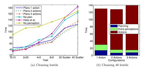
Figure 8: (a) Skill of moving lentils to a container. The results shown are the mean over 5 runs. (b) Time for the case of moving 40 scattered lentils to a container. Extra perceptions include the movements and perceptions needed to tackle occlusions by taking the arm out of the field of view (see Section 4.2.3).
