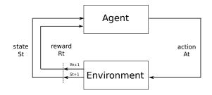
Figure 2: MDP interaction process between an agent and the environment (Figure adapted from [19]).
