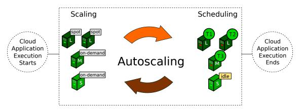
Figure 1: Cyclic autoscaling process that includes the scaling and scheduling subprocesses. L, M and S represent different VM capabilities.  $T_i$  represent tasks to execute.
