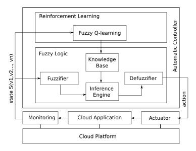
Figure 9: Example of the architecture of a Cloud autoscaling system based on RL and FL. Figure adapted from [78].
