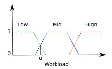
Figure 8: Example of the fuzzy membership function (Y axis) for the workload variable. The fuzzy sets are defined using a trapezoid.
