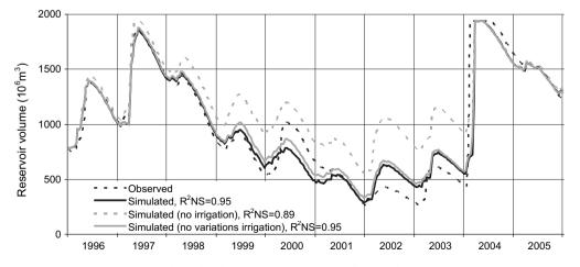
Fig. 6. Observed and simulated reservoir volumes for the Orós reservoir.
