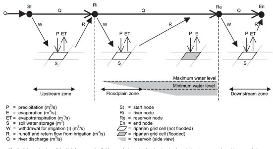
Fig. 2. Schematisation of the link between the field water balance in the riparian lands and the river network and its water balance.
