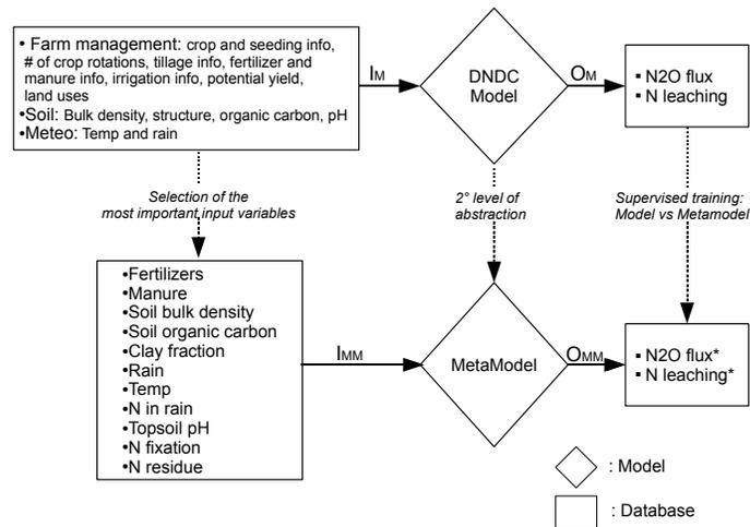
Figure 1: Flow of data through the DNDC-EUROPE model (M) and relationship with the metamodel's one (MM). The input variables of the metamodels were selected from the original DNDC-EUROPE dataset (screening). The estimated (\*) output were compared with the detailed model's output during the training and test phases to improve the metamodel and to evaluate the goodness of the approximation.
