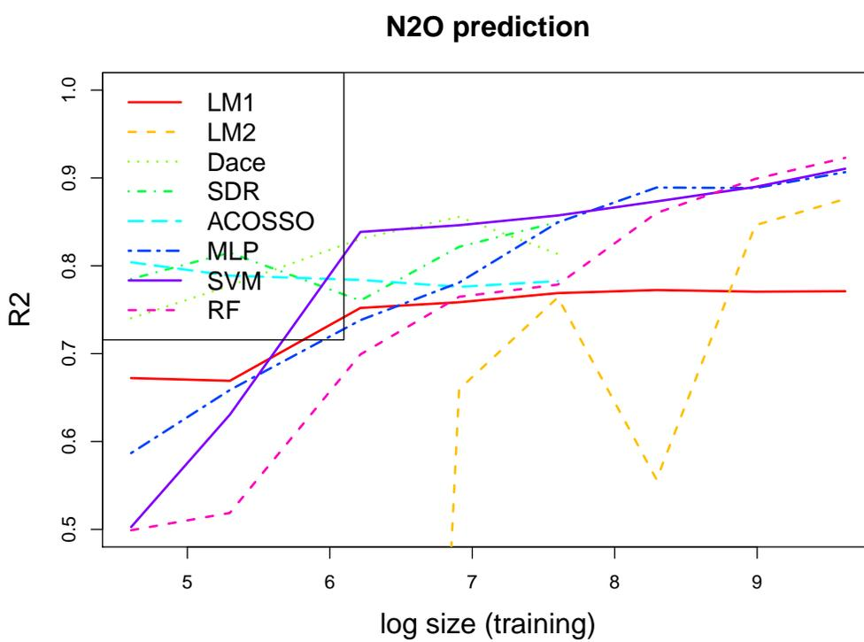
Figure 2:  $R^2$  evolution in function of the size of the train set (log scale) for N<sub>2</sub>O prediction
