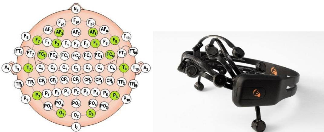
**Figure 1.** A) Emotiv EPOC electrode positioning. B) Emotiv EPOC device.
