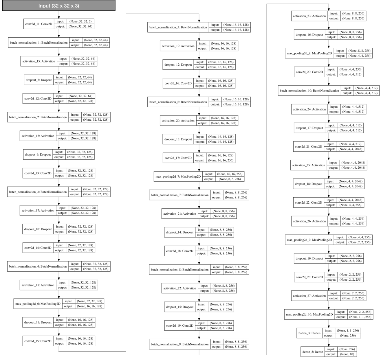
Figure 48: Visualisation of SimpleNet Architecture
