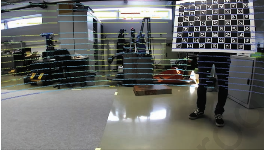
Figure 12: Point cloud projection into the left camera image using the 3D LiDAR to camera calibration. The color represents the points depth. It is worth noting that, this procedure was done using the ATOM full calibration result, with a collection from the test dataset, just like in all the evaluation pipeline. If the system is accurately calibrated, changes in point's color, which denotes a variation of the measured range, should coincide with transitions between far and near objects in the image.
