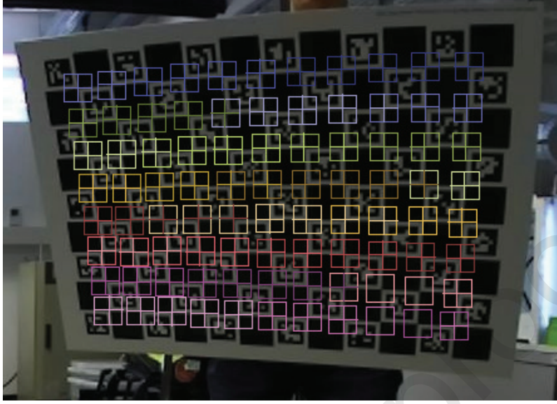
Figure 9: Camera reprojection error from one camera image into the other. Squares represent the expected corner pixel coordinates, and crosses the projected result.
