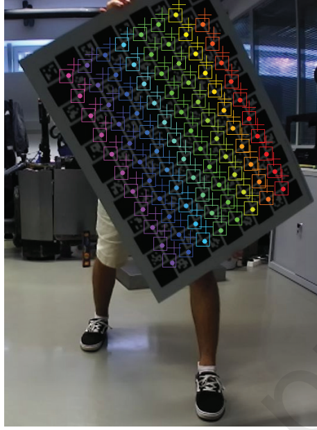
Figure 2: Difference between the initial position of the pattern corners, and the final position of these same projected points, after the optimization has been completed. Squares denote the position of the detected pattern corners; crosses denote the initial position of each projected corner; points denote the current position of the projected points.
