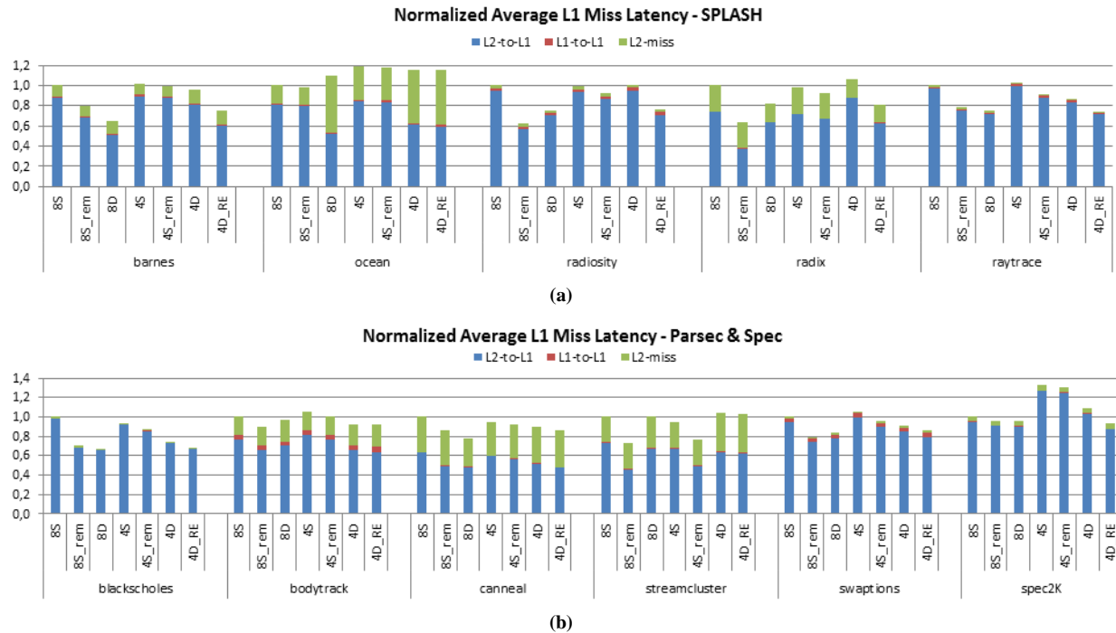
Figure 12: Breakdown of the normalized average L1 miss latency, for SPLASH (a) and Parsec & Spec applications (b), with respect to the components L2 miss (green), L2 hit that determines a transfer from L2 to L1 (blue), and L2 hit that determines a transfer from L1 to L1 (red).
