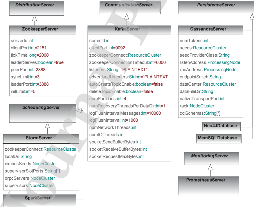
Figure 6: Specialization of PlatformServer classes for Apache-based implementation
