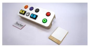
Figure 4. Photo-sorting Console with RFID card & reader
