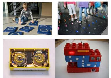
Figure 3. Playware, and modular tiles (up), I-BLOCKS (down) are examples of manipulative technology and modular robotics (photos courtsey of H. Lund).
