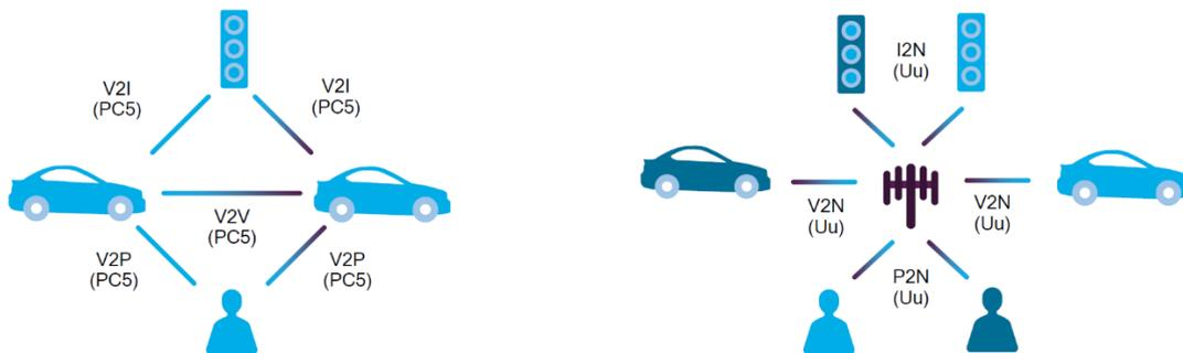
Fig. 5. C-V2X modes: (a) direct communications; (b) network communications
