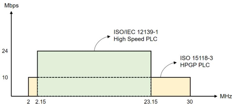
Fig. 2. Frequency band overlap between the PLC standards
