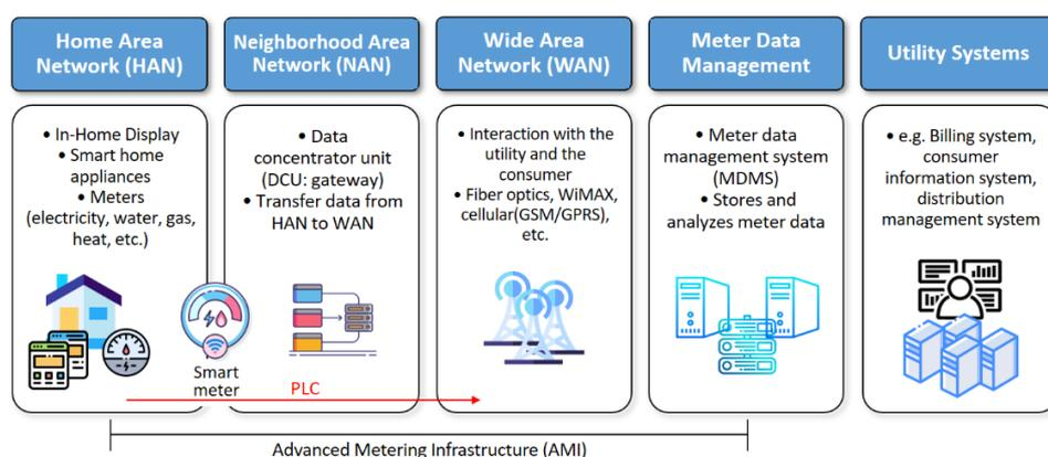
Fig. 1. Components and communications of an AMI
