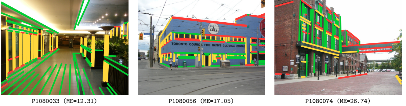
Figure 4: A sample of the worst RPA results on vanishing point detection . Lines incident to the same vanishing points are represented with the same color.
