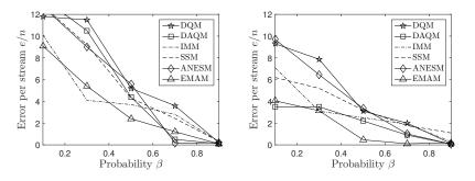
Figure 8: Impact of probability  $\beta$  on error per stream e/n for AVG operator over DQM, DAQM (a = 0.95, c = 0.5), IMM, SSM, ANESM, and EMAM, using n = 54 context streams and (left) h = 10, (right) h = 50; Intel Lab Data.
