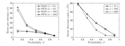
Figure 1: (Left) Error per stream e/n for AVG operator and (right) percentage  $\nu\%$  of the DQM and the SWM against probability  $\beta$ .
