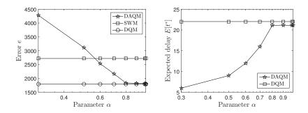
Figure 5: (Left) Error e and (right) expected delay  $E[t^*]$  against a of the DAQM and the DQM for AVG operator with  $\beta = 0.5$ ;  $c = 0.5\lambda$ .
