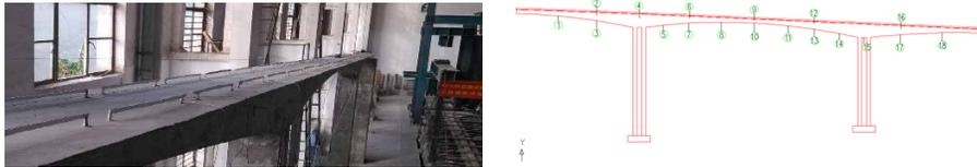
Figure 6: Sensor placement on the scale model of TCRF Bridge.
