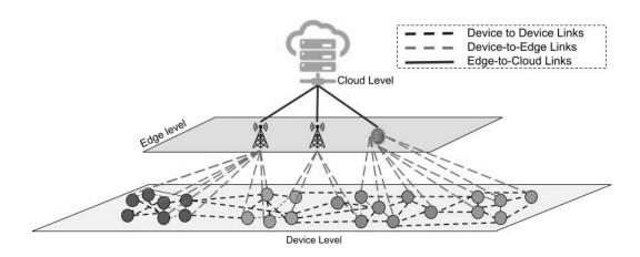
Figure 1: Network topology including Edge network levels and communication links.
