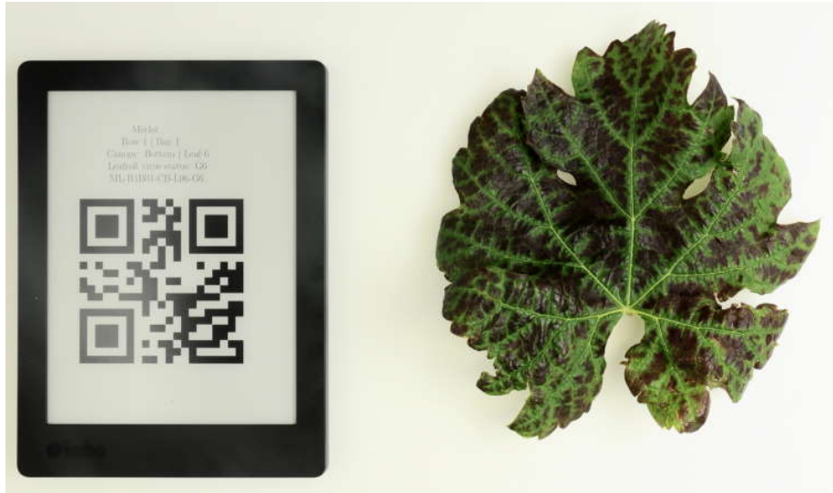
Figure 7: Quick response (QR) code being used in scientific imaging under controlled conditions. An e-reader containing a pre-generated PDF document displays a unique QR code along with human-readable text for each grape leaf being imaged. The QR code contains the character string ‘ML-R1B01-CB-L06-G6’, which indicates the variety, location and virus status of the grapevine from which the leaf was taken, as well as the position on the vine and number of the leaf itself.
