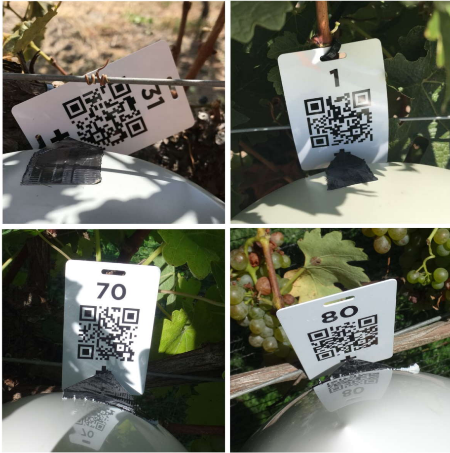
Figure 12: Examples of misread QR codes in images captured in a trial in grapevines testing the accuracy of a precise global navigation satellite system (GNSS). Possible explanations for read failure are occlusion (top-left), distortion or reflection (top-right), contrast (bottom-left), and perspective warp (bottom-right).
