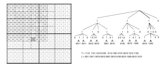
Figure 1: Example of  $k^2$ -tree for a binary matrix using k = 2.
