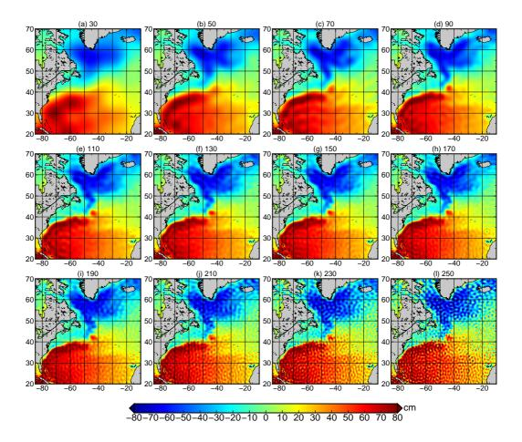
Figure 1: The mean dynamic topography (MDT) of the North Atlantic, based on the CLS01 mean sea surface and the 3rd generation GOCE time-wise gravity model, with truncations of the spherical harmonic expansion of the MDT ranging from L = 30 to 250 in intervals of 20.
