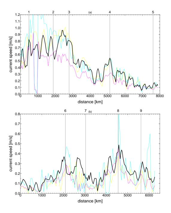
Figure 8: (a) Current speeds along the warm path marked in Figure 4d with current speeds given by the unfiltered L = 170 GOCE MDT shown in Figure 2h (black), the CLS09 MDT (yellow), the MAX11 MDT (magenta) and the NMM03 MDT (cyan). (b) Repeating (a) but for the cold sub-polar path marked in Figure 4d. The vertical lines correspond to the positions marked on Figure 4d.
