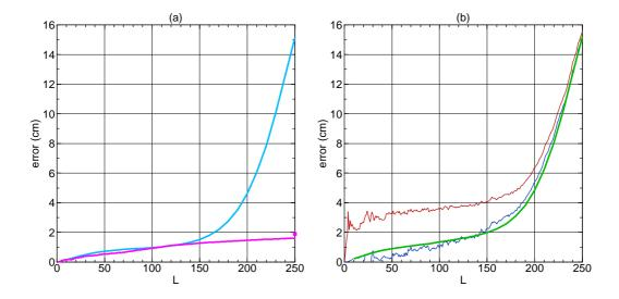
Figure 5: (a) North Atlantic mean formal errors for the geoid obtained from the third GOCE timewise gravity model (cyan). An informal estimate of the CLS11 MSS error based on the RMS difference between it and the DTU10 MSS (magenta). The area mean over the North Atlantic of the supplied CLS11 formal error field is marked by the solid square. (b) Upper (red) and lower (blue) bounds on the GMDT commission error (repeated from Figure 3a). The quadratic sum of the geoid and MSS errors (green).
