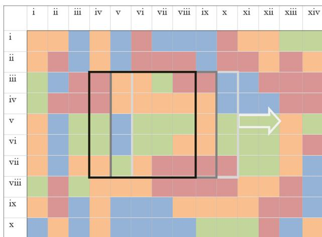
**Fig. 2.** KRC example of a  $5 \times 5$  pixel window applied on a  $14 \times 10$  pixel image classified into 4 classes (depicted in different colours). Based on the similarity index between  $5 \times 5$  window and the training adjacency event matrices, KRC will assign to each pixel the thematic habitat class for which the similarity index is maximum (Keramitsoglou et al., 2006).
