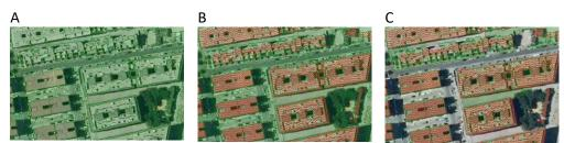
Figure 6. (1.5 columns) Integration of image segmentation and LiDAR. A: Segmentation polygon layer. B: LiDAR points classified as buildings (red dots) superimposed on the segmentation. Points can be seen only on the roofs. C: Selection of segments containing building points.
