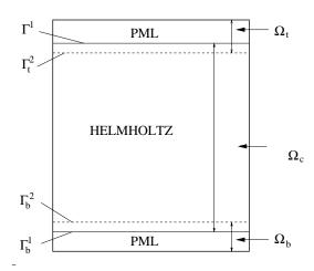
Figure 1: Domain decomposition into three overlapping subdomains
