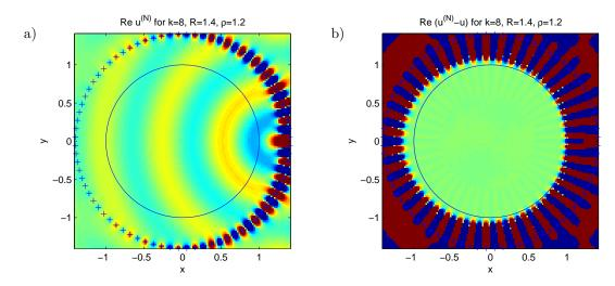
Fig. 4. MFS approximation to the interior Helmholtz BVP in the disc with given boundary data corresponding to a single source (39) outside the domain at  $\rho = 1.2$ , with N = 80 and R = 1.4. a) Re  $u^{(N)}$ , b) residual Re  $(u^{(N)} - u)$  on a color scale  $3 \times 10^4$  times more sensitive than a).
