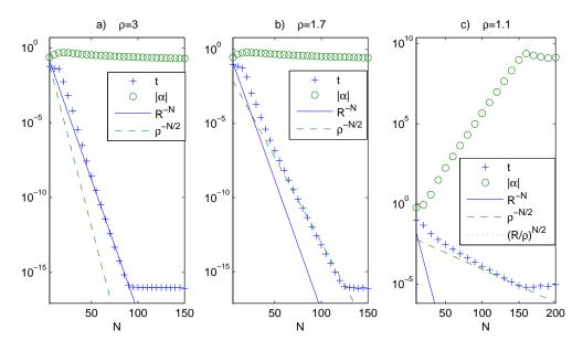
Fig. 3. Convergence and coefficient sizes as a function of N, for the MFS approximation to the interior Helmholtz BVP in the unit disc given boundary data corresponding to a single source (39) at radius  $\rho$ . The wavenumber is low (k = 8). The MFS sources are at R = 1.5. For visual comparison the relevant power laws from Theorems 3 and 7 are shown (sometimes the constants have been chosen to match the data). There were M = 240 boundary points.
