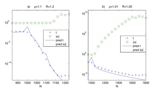
Fig. 5. Convergence and coefficient sizes as a function of N, for MFS approximation to the interior Helmholtz BVP in the disc at high wavenumber k = 500. The boundary data corresponds to a single source (39) outside the unit disc at radius  $\rho$ , with MFS sources at R. For a)  $\rho = 1.1$ , R = 1.2, b)  $\rho = 1.01$ , R = 1.05. The 'predicted' curves are given by (42) using (41), with (45) modeling both  $\hat{s}(m)$  and  $\hat{v}(m)$ .
