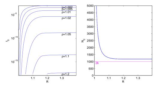
Fig. 6. a) (left plot) Minimum achievable boundary error norms  $t_0$  and b) (right plot) corresponding basis sizes  $N_0$ , predicted for a selection of source radii  $\rho$  and MFS source point radius R, for the Helmholtz BVP in the unit disc at high wavenumber k = 500. The predictions are done in the range  $R > \rho$  using the model in Sec. 2.4. Note that in b) all the graphs for different  $\rho$  lie on top of one another.
