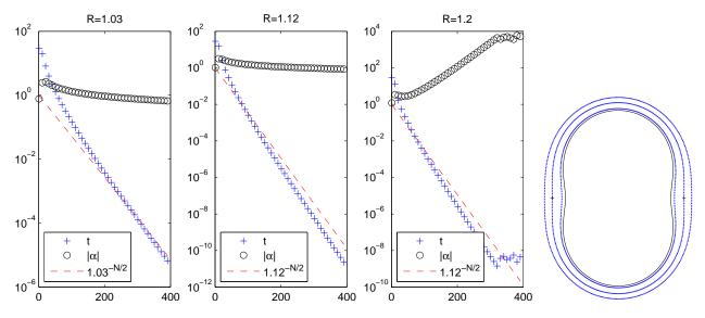
Fig. 9. Left three plots: Estimated (dashed lines) and observed ('+') rates of convergence of the MFS on the inverted ellipse for charge points with conformal radii R = 1.03, R = 1.12 and R = 1.2. The corresponding coefficient norms  $|\alpha|$  are denoted by 'o'. Right plot: Domain and positions of the charge points (shown as dots) for the above three conformal radii, with branch-type singularity locations ('+' signs).
