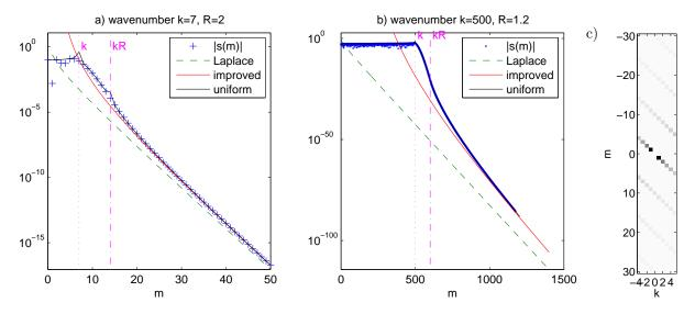
Fig. 2. Comparison for the unit disc of layer-potential eigenvalue magnitudes  $|\hat{s}(m)|$  given in (12) against various asymptotic expressions: 'Laplace' (14), 'improved' (44), and 'uniform' (45). a) low wavenumber, b) high wavenumber. Panel c) shows density plot of matrix elements (20) of Q for N = 10, in the domain  $|m| \leq 30$ . In c) we chose unrealistically small values of R and k in order to make the super- and sub-diagonals more visible.
