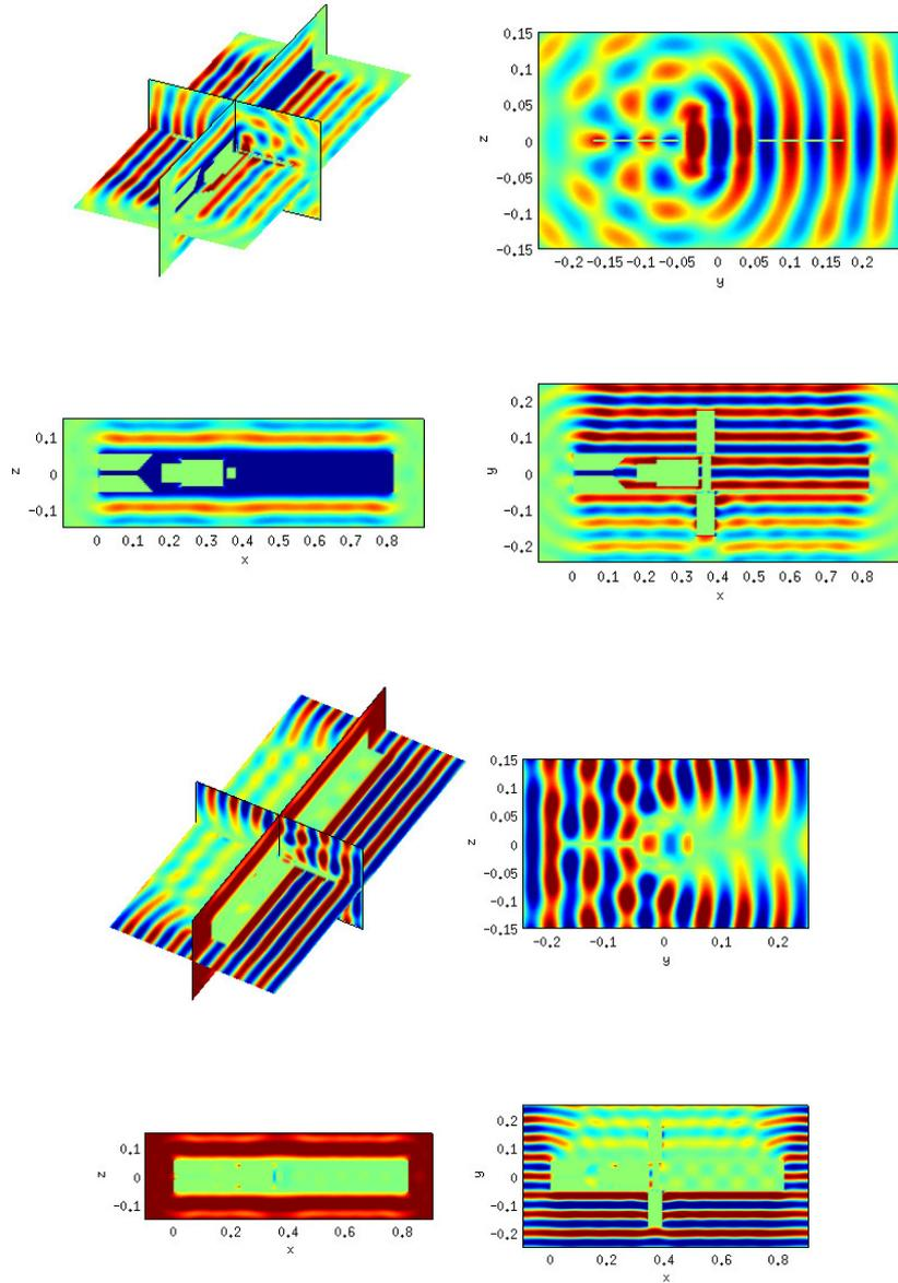
Figure 15: On top, real part of diffracted field  $E_x$ , and on bottom the total field. Scattering by a satellite
