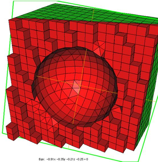
Figure 10: Example of hybrid mesh used for the scattering by a sphere
