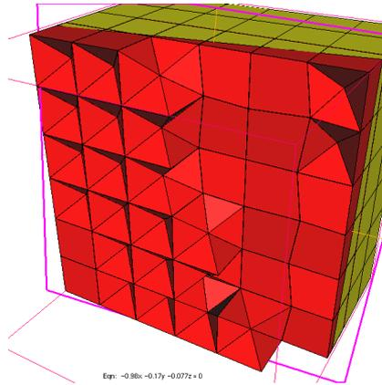
Figure 7: Pyramidal mesh used for the dispersion analysis.
