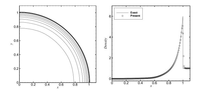
Figure 3. Two-dimensional Sedov problem: (left) 10 density contours from 0 to 6; (right) density profile along y = 0.
