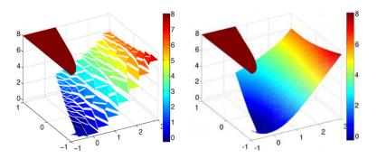
**Fig. 4.11.** WG solutions of Example 8. Left: Mesh level 1; Right: mesh level 5.
