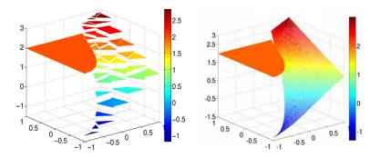
**Fig. 4.10.** WG solutions of Example 7. Left: Mesh level 1; Right: mesh level 5.
