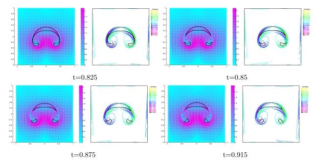
Figure 6.8: The flow field (with arrows representing the velocity vectors and color representing the norm value) and vorticity contours for the rising drop with density ratio 1: 50 from t=0.825 to t=0.915  $\rho_1=1, \rho_2=50, \ \epsilon=0.01, \ C=200\epsilon^2, \ M=1/(20\epsilon), \ Pe=1000/\epsilon, \ 1/Fr^2=10$  and  $\Delta t=0.00025$ .
