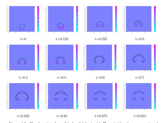
Figure 6.5: The drop interfaces (black solid line) with  $\nabla \cdot \mathbf{u}$  (with color representing the value distribution) for the rising drop with density ratio 1 : 50,  $\rho_1 = 1$ ,  $\rho_2 = 50$ ,  $\epsilon = 0.01$ ,  $C = 200\epsilon^2$ ,  $M = 1/(20\epsilon)$ ,  $Pe = 1000/\epsilon$ ,  $1/Fr^2 = 10$  and  $\Delta t = 0.00025$ .
