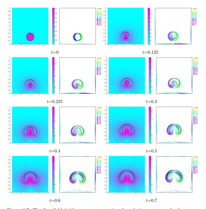
Figure 6.7: The flow field (with arrows representing the velocity vectors and color representing the norm value) and vorticity contours for the rising drop with density ratio 1:50 from t=0 to t=0.7.  $\rho_1=1, \rho_2=50, \epsilon=0.01, C=200\epsilon^2, M=1/(20\epsilon), Pe=1000/\epsilon, 1/Fr^2=10$  and  $\Delta t=0.00025$ .
