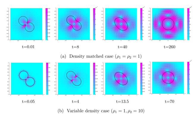
Figure 6.1: The deformed drop interfaces (black solid line) with the velocity fields (with arrows representing the velocity vectors and color representing the norm value) for kissing drops.  $\epsilon = 0.01$ ,  $C = 100\epsilon^2$ ,  $M = 1/(10\epsilon)$ ,  $Pe = 100/\epsilon$  and  $\Delta t = 0.01$ .
