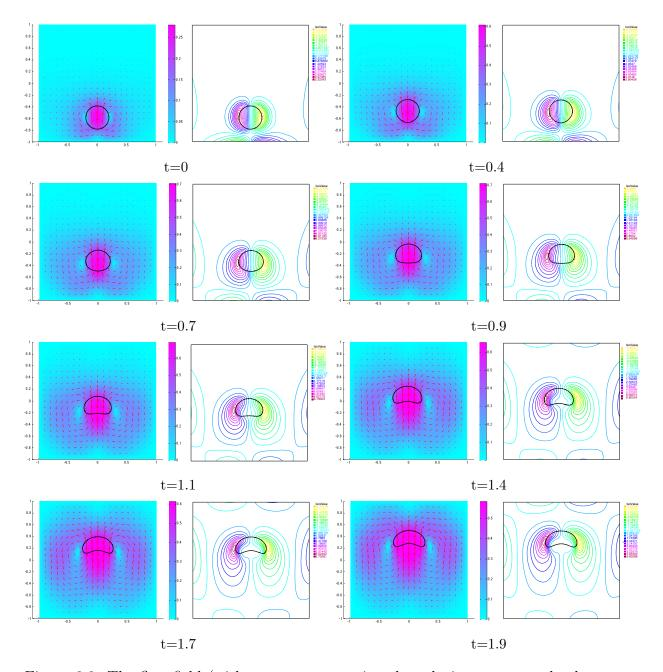
Figure 6.6: The flow field (with arrows representing the velocity vectors and color representing the norm value) and vorticity contours for the rising drop with density ratio 1: 2,  $\rho_1 = 1$ ,  $\rho_2 = 2$ ,  $\epsilon = 0.01$ ,  $C = 200\epsilon^2$ ,  $M = 1/(20\epsilon)$ ,  $Pe = 1000/\epsilon$ ,  $1/Fr^2 = 10$  and  $\Delta t = 0.001$ .
