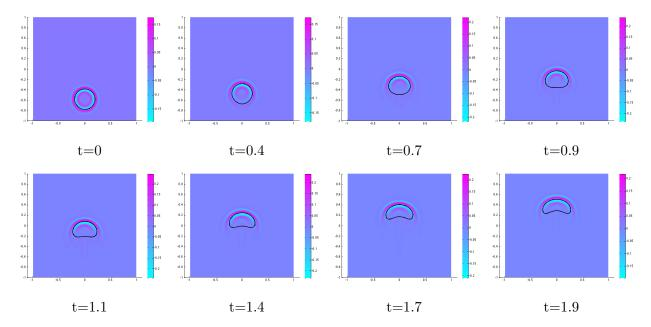
Figure 6.4: The drop interfaces (black solid line) with  $\nabla \cdot \mathbf{u}$  (with color representing the value distribution) for the rising drop with density ratio 1 : 2,  $\rho_1 = 1$ ,  $\rho_2 = 50$ ,  $\epsilon = 0.01$ ,  $C = 200\epsilon^2$ ,  $M = 1/(20\epsilon)$ ,  $Pe = 1000/\epsilon$ ,  $1/Fr^2 = 10$  and  $\Delta t = 0.00025$ .
