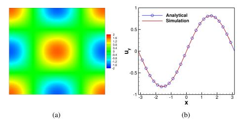
Figure 3: (a) The vorticity contour plot for Taylor-Green vortices at time T = 10. (b) Cross-section of the velocity y-component profile at the horizontal center line for Taylor-Green vortices at time T = 10.
