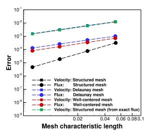
Figure 4: The numerical convergence of the velocity 1-form (flux) and the interpolated velocity vector for the Poiseuille flow test case. The dashed lines represent the 1-st and 2-nd order slopes.
