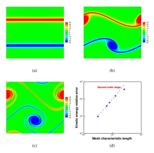
Figure 5: The vorticity contour plot for double periodic shear layer with a mesh of 204800 elements at time: (a) T=0.0, (b) T=0.8 and (c) T=1.2. (d) The convergence of the relative kinetic energy error  $(\frac{KE(0)-KE(T)}{KE(0)})$  with the characteristic mesh length at simulation time T=2.0. The dashed red line represents the second order slope.
