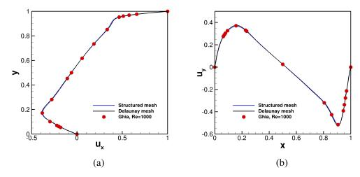
Figure 2: Cross-section of the velocity profile at the two domain center lines for driven cavity test case at Reynolds number = 1000.
