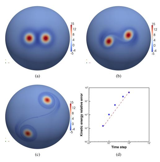
Figure 7: The vorticity contour plot for two Taylor vortices on a spherical surface meshed with 327680 elements at time: (a) T=0.0, (b) T=2.0 and (c) T=10.0. (d) The convergence of the relative kinetic energy error with the time step at simulation time T=10.0. The dashed red line represents the second order slope.
