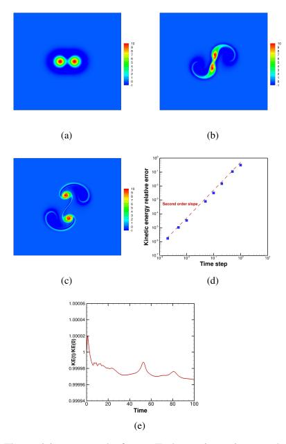
Figure 6: The vorticity contour plot for two Taylor vortices using a mesh consisting of 132204 elements and a time step  $\Delta t = 0.005$  at time: (a) T=0.0, (b) T=3.0 and (c) T=5.0. (d) The convergence of the relative kinetic energy error with the time step at simulation time T=20.0. The dashed red line represents the second order slope. (e) The evolution of the relative kinetic energy with time for two Taylor vortices on a hexagonal domain.
