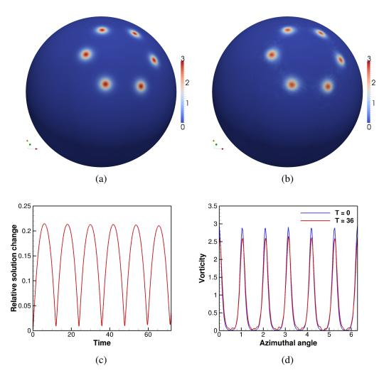
Figure 8: The vorticity contour plot for 6 vortices on a spherical surface at latitude  $\theta=0.4$  at time: (a) T=0.0 and (b) T=36.0. (c) The relative solution change  $(\frac{\|U(t)-U(0)\|}{\|U(0)\|})$  versus the simulation time. (d) The vorticity strength along a circle at latitude  $\theta=0.4$ .
