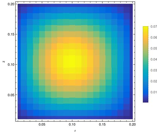
Figure 8:  $E_\phi$  for the fundamental eigenmode in the plasma-filled cylindrical cavity.
