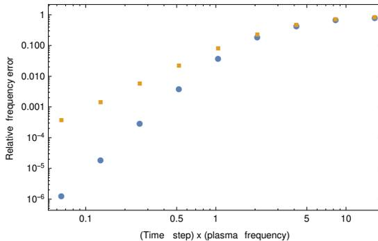
Figure 7: Error on the numerically determined fundamental frequency of a cylindrical plasma-filled cavity, determined with the second-order (orange) and fourth-order (blue) methods.
