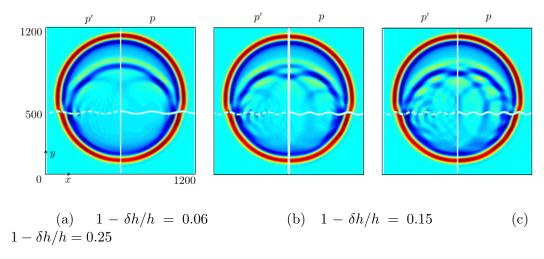
Figure 16: Wavefields for a curved mean line  $\Gamma$ . Expect the shape of  $\Gamma$ , the calculations are identical to those of Fig. 12 for  $f_0 = 10$  Hz. On (a-c), the left panels show the wavefields  $p^r$  in the real problem (with dotted white lines indicating  $\Gamma$ ); the right panels the wavefields p in the homogenized problem (with the white region indicating the homogenized interface.
