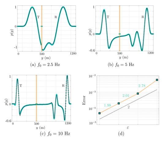
Figure 13: (a-c) Pressure profiles along the centerline x = 600 m from Figs. 12,  $p^{\rm r}$  (blue symbols) and p (black lines). (d) Error  $|p^{\rm r} - p|/|p|$  calculated on the transmitted wave  $y \in [0490]$  m as a function of  $\varepsilon = 2\pi f_0/c$  (an extra point at  $f_0 = 20$  Hz has been considered); dotted grey line shows the  $\varepsilon^2$  law.
