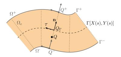
Figure 4: Parametrization of  $\Gamma$  with the parameter s; the vectors  $(\mathbf{n}, \boldsymbol{\tau})$  locally normal and tangent to  $\Gamma$  at  $Q_{\Gamma}[X(s), Y(s)]$  are also normal and tangent to  $\Gamma^{\pm}$  at  $Q^{\pm}$  by construction.
