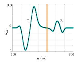
Figure 11: Pressure profiles along the slice in dotted line in Fig. 10(b), of the reference (black line) and numerical (open symbols) homogenized solutions; the agreement between both is  $0.5\%_0$ .
