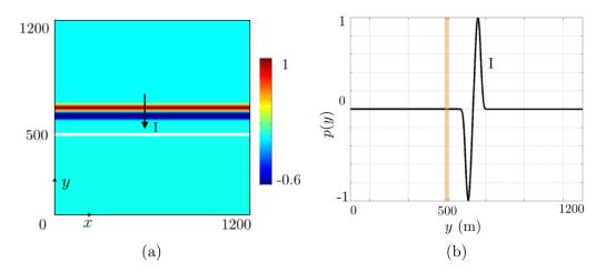
Figure 6: (a) Pressure field of the incident wave (for the reference solution) imposed at the initial time of the simulation and (b) corresponding y- profile.
