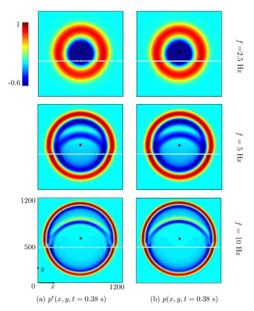
Figure 12: Pressure fields  $p^{\rm r}$  (real problem with the array) and p (homogenized problem) computed with ADER 4 at t = 0.38 s for  $f_0 = 2.5$ , 5 and 10 Hz.  $f_0$  is the central frequency of the signal h(t) in (40) imposed by the source point (indicated by the black point).
