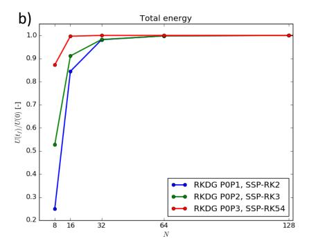
Fig 9a shows the electromagnetic energy after one periodic orbit as a function of number of zones along one direction of the twodimensional mesh for P=1, P=2 and P=3 DG schemes. Fig. 9b shows the same information for P0P1, P0P2 and P0P3 schemes. Fig. 9c shows the same information for P1P2 and P1P3 schemes. All second order schemes are shown in blue; all third order schemes are shown in green; all fourth order schemes are shown in red.
