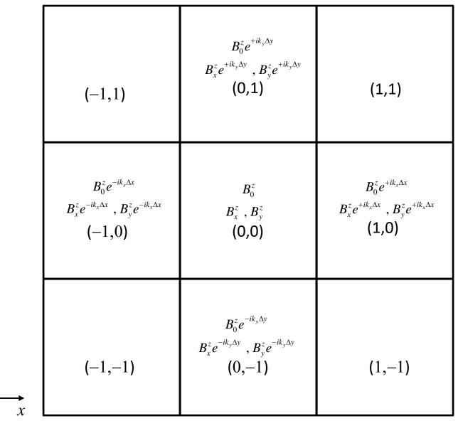
Fig. 2a shows how the facially collocated Fourier modes associated with the electric displacement relate to one another across the different faces of the mesh. Fig. 2b shows the analogous information for the Fourier modes associated with the magnetic induction. These Fourier modes are used in making the von Neumann stability analysis.
