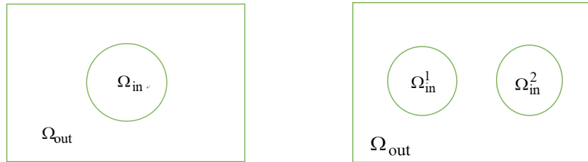
Figure 2.1: The division of \Omega into atomic spheres \Omega_{\text{in}} and a interstitial region \Omega_{\text{out}} .
