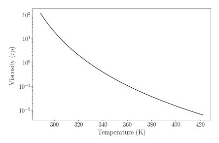
Figure 1: The Bennison viscosity correlation for heavy oil.
