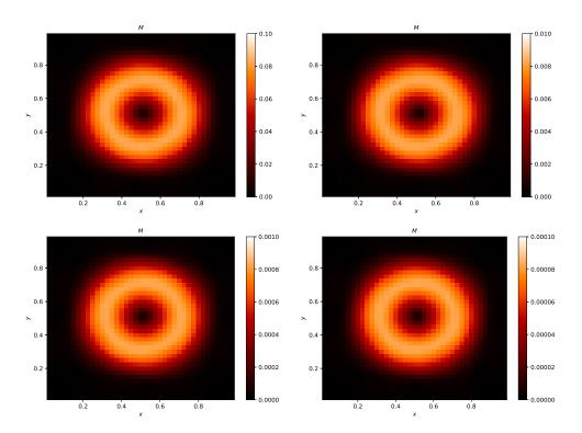
Figure 3: Mach number distribution for different maximal Mach numbers at t=1. Top left:  $M=10^{-1}$ . Top right:  $M=10^{-2}$ , bottom left:  $M=10^{-3}$ , bottom right:  $M=10^{-4}$
