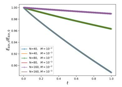
Figure 4: Loss of kinetic energy for different grids and Mach numbers after one full turn of the vortex (non-dimensional).
